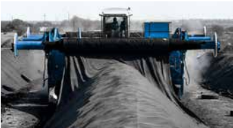
Professional optimization of the composting process – BACKHUS Fleece Winder
