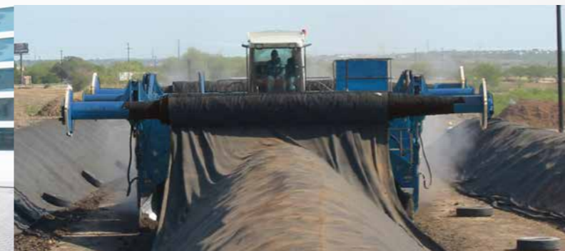
Professional optimization of the composting process - BACKHUS Fleece Winder
