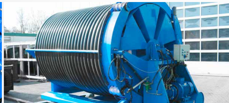
BACKHUS HD S, Radio controlled - hose drum with 3" or 4" connection
