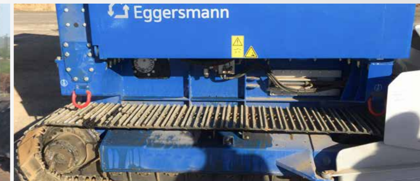
For increased traction on loose ground - the landfill undercarriage
