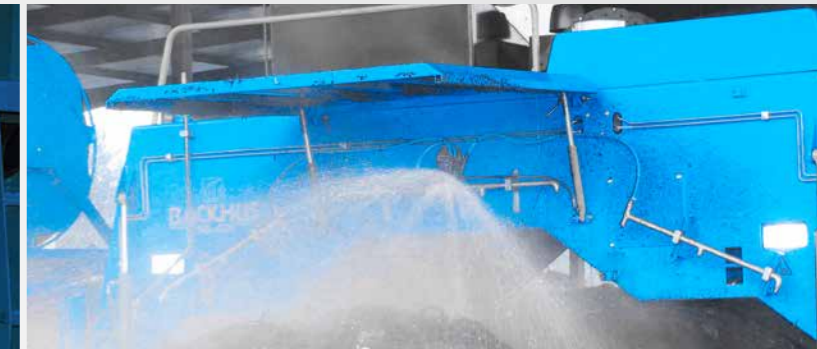
Process optimization - injecting water during turning
