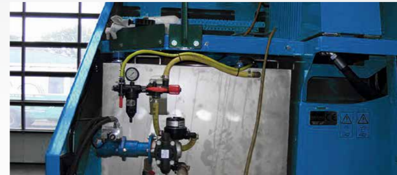
Concentrate injection for process optimization - for fast composting
