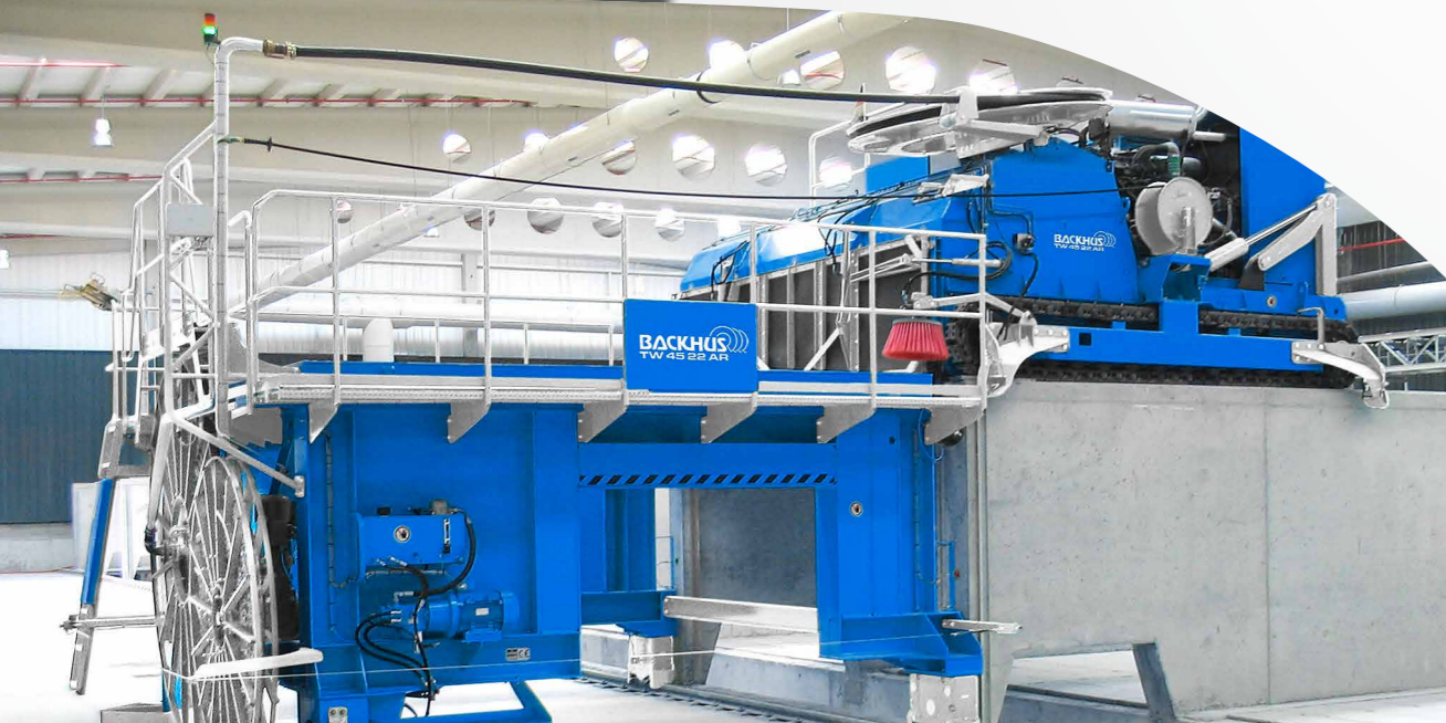
Transfer waggon / platform
