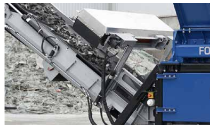
Hydraulically adjustable magnet (also F 38)
