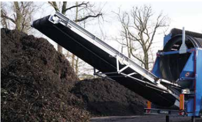
Extended coarse grain conveyor, discharge height up to 3,800 mm
