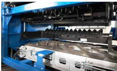
After breaker bars replaceable within 10 minutes (also F 38)
