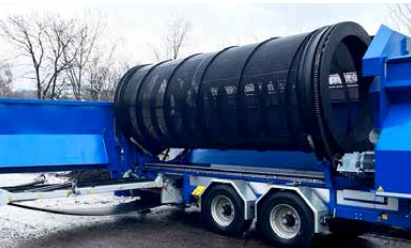
Quick and easy changing of the screening trommel
