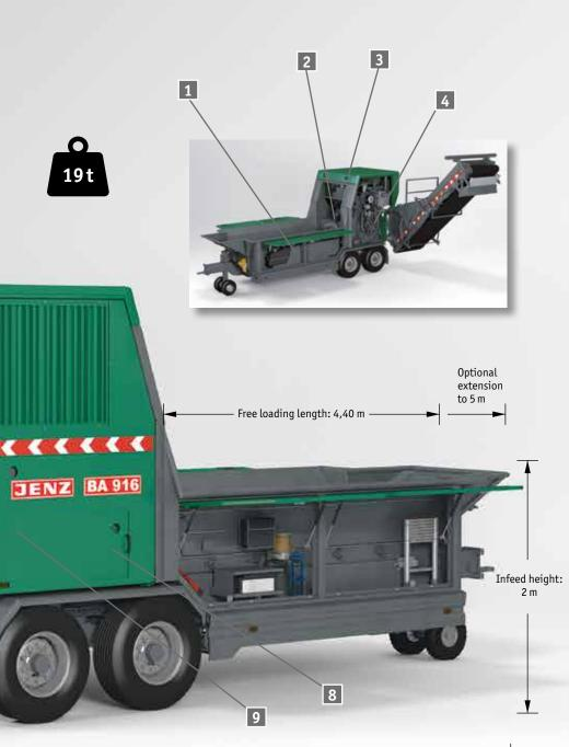
Transport position: 10,40 m (overall combination length with 3-axle HGV less than 18.75 m)
