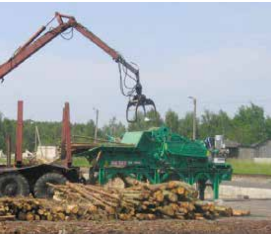
2. Aggressiver Einzugs: 800 – 1000 mm Aggressive infeed: 800 – 1000 mm
