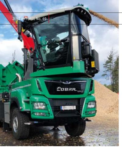
level V to power the chipper by itself-without AdBlue, by the way. This also means that the motor is spared when it is not chipping, e.g. during transport. In addition, the 32-tonne chipper surprises users with its enormous manoeuvrability thanks to the MAN 8x4-4 carrier vehicle, so that even operations away from the industry are not a problem. Those who need even more flexibility can also switch to AGRO tyres.
