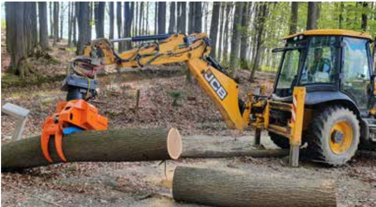
Sturdy and low-wear woodgripper with saw unit.
