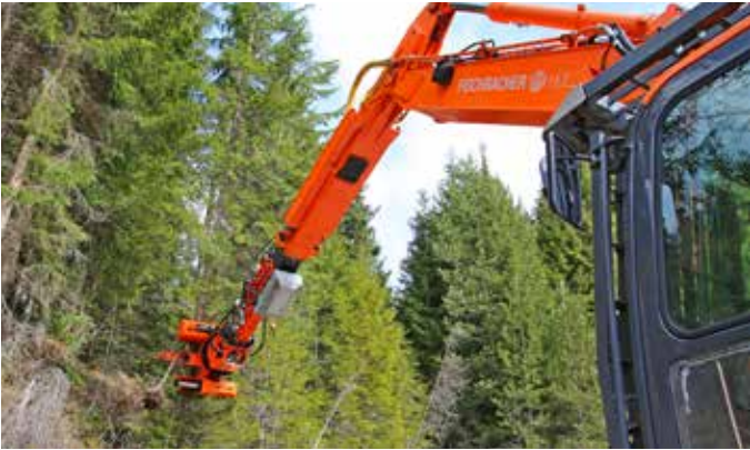
Attachment coupler with Woodcracker® C250.
