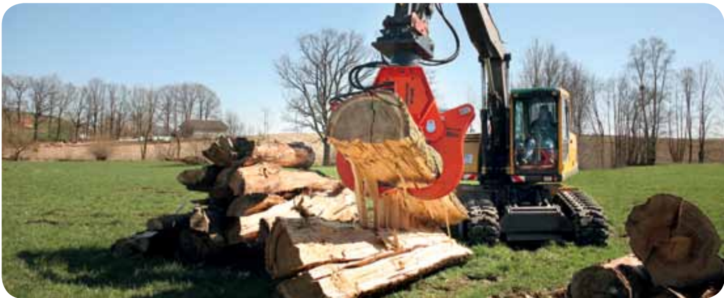
Woodcracker® W for splitting thick trunks.
