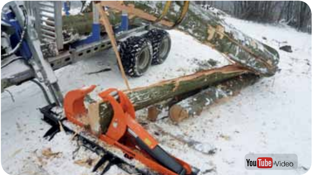
Woodcracker® L for splitting thick trunks.
