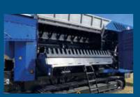
Comb door - can be opened hydraulically = free access to shredding area
