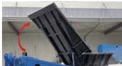
Large volume, tiltable hopper (SE 25)
