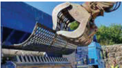
Screen basket system for defined final particle size
