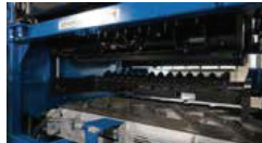
Secondary crushing beam can be changed within 10 minutes (also SE 25)
