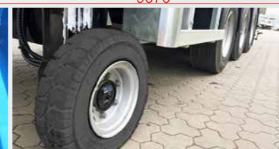
Drive unit – allows to move the machine using the radio remote (Semi-trailer only)
