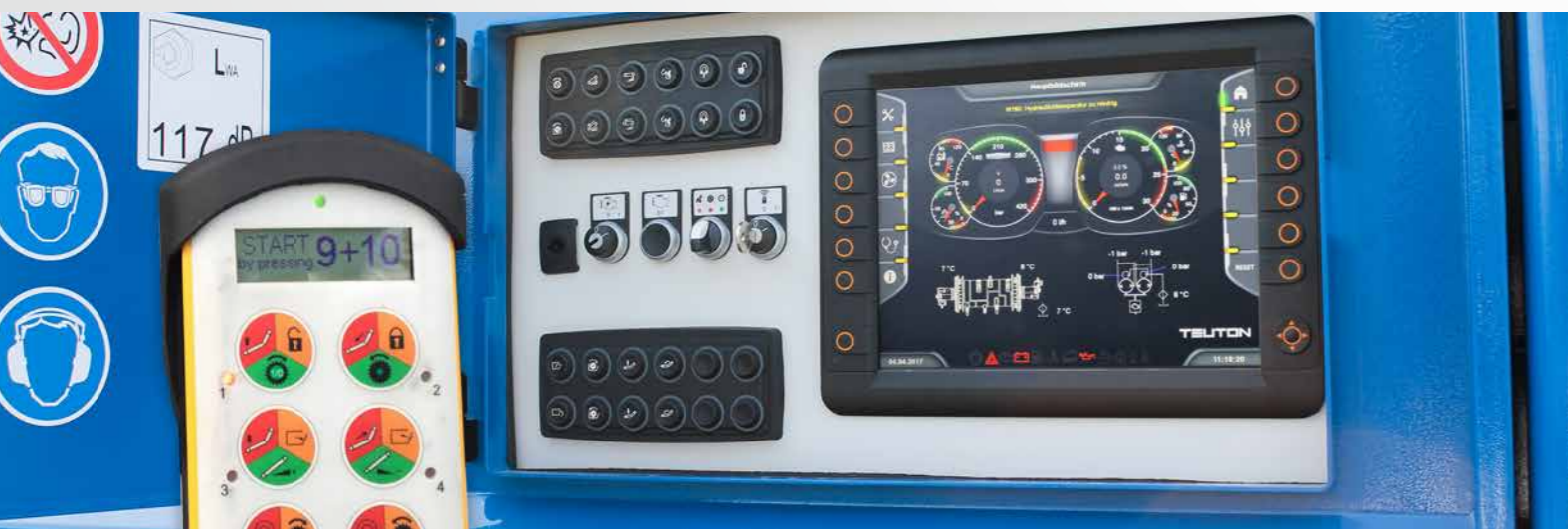
IFM controls with 12.1" touch panel + radio unit with display
