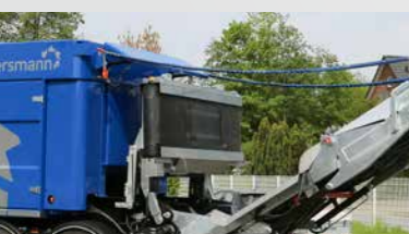
Hydraulic adjustable overbelt neodym magnet
