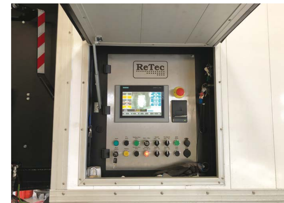
Integrated touch weight- and control panel for plant.
