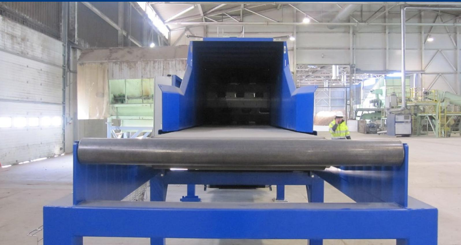
The solution was simply to install the ReTec bale-opener in front of the existing drumscreen-opener, and convert it to a conventional drum-screen. With the SRF completely loosed, the screen can now very effectively screen the wrapping from the fluff. The output is very clean and homogenous flow of fluff, and the waste fraction is very pure, i.e. contains very little SRF.
