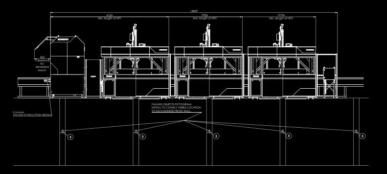
The delivery of a complete Heavy Picker system includes a sensor unit, a control system, 1 to 3 robot arms, chute collars and a safety cage.
