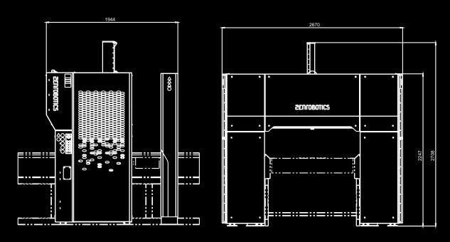
The delivery of a complete Fast Picker system includes a sensor unit, control system, robot arm, suction gripper, and safety panels.
